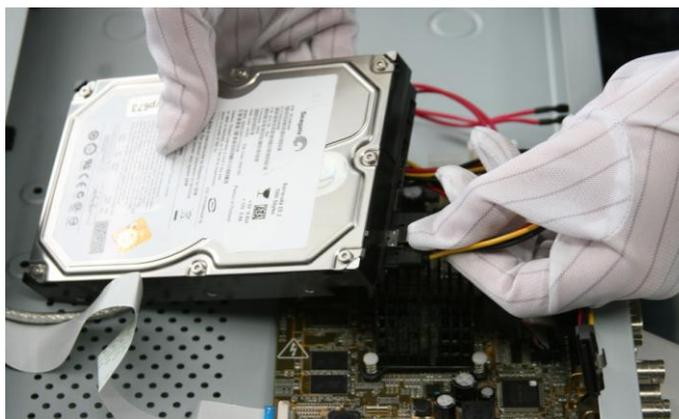
4. Place the HDD on the bottom of the device and then fasten the screws on the bottom to fix the HDD.
