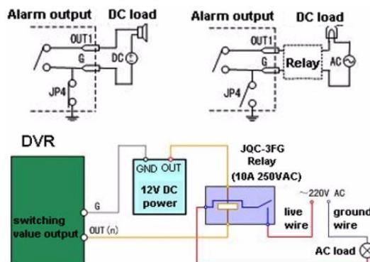
For DC load, JP4 can be used within the limit of 12V/1A safely. If the interface is connected to an AC load, JP4 should be left open. Use an external relay for safety (as shown in the figure above).
