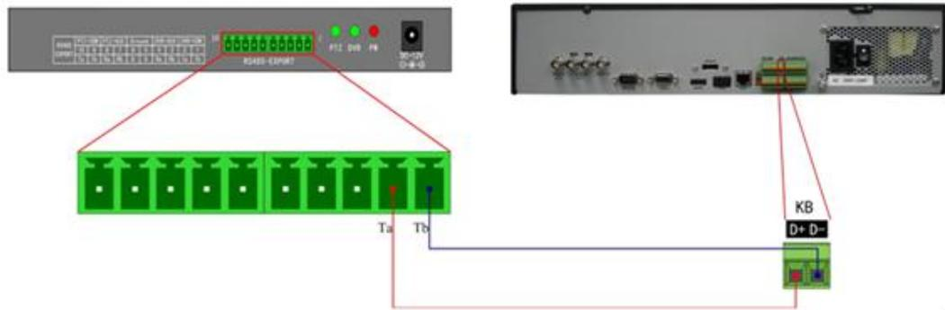
To connect a controller to the NVR:
