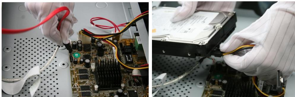
3. Connect the power cable to the HDD.
