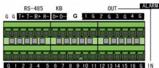
The alarm input is an open/closed relay. If the input is not an open/closed relay, follow the connection diagram below:
