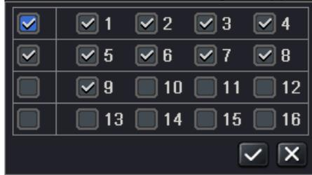
Take 16-channel DVR for example: user can tick off 16 channels form 1-ch to 16-ch at random to display the live pictures. Then click  button to confirm the setting.
