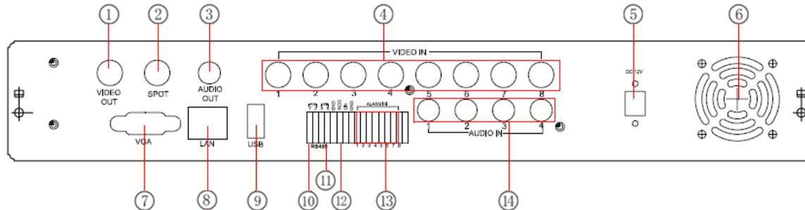
Fig 2.6 Rear Panel for 8-ch
