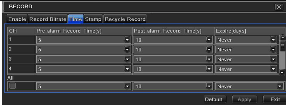
Fig 4-13 record configuration-time
